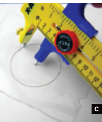
Fig. A: Calipers give an accurate inner diameter of your yo-yo. Fig. B: Set the compass cutter to match the inner radius. Fig. C: Cut the side cap out of sheet plastic. Fig. D: Measure your coin cell battery, then lightly scribe
