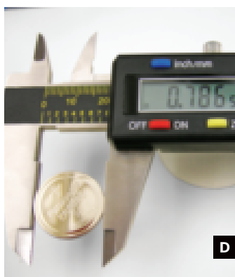
Fig. A: Calipers give an accurate inner diameter of your yo-yo. Fig. B: Set the compass cutter to match the inner radius. Fig. C: Cut the side cap out of sheet plastic. Fig. D: Measure your coin cell battery, then lightly scribe
