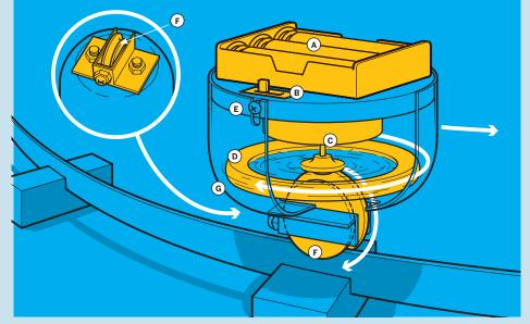
A Three AAA **batteries** power the Gyrocar's motor for 30+ total minutes.
