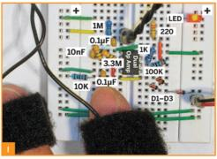
**2e.** For final amplification, so that the output voltage will cross the LED's threshold with signal spikes, a  $100 k\Omega$  resistor sets the op-amp's amplification very high. If the circuit is too sensitive to GSR and the LED flashes too often, swap the resistor between the amp's (–) input and output for a  $10 k\Omega - 20 k\Omega$ , or use a potentiometer if you want more control.
