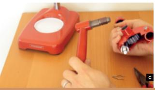
Disassembling the juicer. First, remove the coneshaped cup from the juicer shaft (save it — it may come in handy for a future project). Figs. A and B: Remove the lever assembly.
