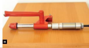
and the piston mounting thread. Figs. G and H: Juicer shaft, coupler, and piston shown separately and joined together.
