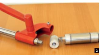
Connecting the juicer shaft to the actuator piston. Fig. E: Cut a 1½" length of 1" aluminum rod. Fig. F: Drill and tap the rod to couple the juicer shaft
