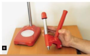
Fig. C: Use pliers to remove the retention clip on the lever handle. Fig. D: Place the down-shaft at its highest point, and reinsert the lever handle at the starting angle, as shown here.
