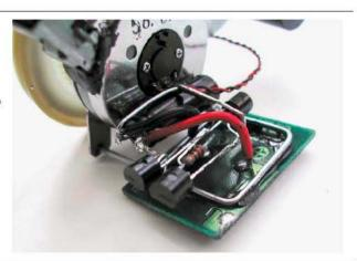
3j. Finally, connect the motor. Solder the positive/red motor wire onto the 3906 emitter (left) pin and the negative/black wire to the 3904 collector.
