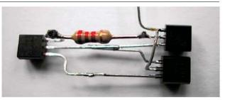
1d. If you're making both BEAMbots, build a second Solarengine circuit by repeating steps 1a-1c above. From here, you can continue on to step 2 to build a Trimet, or jump ahead to step 3 and build a Solarroller.
