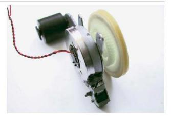
3d. Cut about 4" of wire from a large paper clip and fashion it into a U shape. For the Solarbotics motor, it can be just wide enough to run between the two upper mounting holes. Trim the remaining piece of paper-clip wire and solder it across the U as a cross-brace, about 3/4" from the open end.
