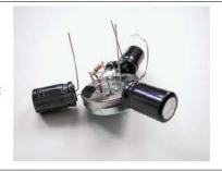
2d. The motor case is our circuit's ground (-); now let's work on the power (+) side. Take a small paper clip and bend it into a ring with the same diameter as the motor. (Conveniently, Walkman motors are the size of a quarter, so you can use one as a form to bend the clip around.) When you have a decent circle, solder it together.
