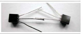
1b. Use needlenose pliers to gently bend the 3904 emitter pin (left) 90 degrees to the side and its collector (right) 90 degrees up. Bend the 3906 base pin (middle) 90 degrees up and its emitter (left) 90 degrees to the side. Solder the 2.2kΩ resistor from the 3904 collector to the 3906 base.
