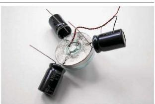
2c. Center the circuit assembly over the motor, and solder a scrap lead from the 3904 emitter to the motor casing. This grounds the circuit, while also attaching it to the motor. For optimal balance, bend this connecting wire at 90 degrees, and try to position the circuit in the middle of the motor.
