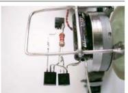
3h. Turn the Solarengine upside down and solder a scrap component lead to the 3904 emitter pin at the point where it attaches to the 1381 trigger's Pin 3. Bend the capacitor's negative/cathodelead around the undercarriage side of the cap's barrel, and solder it to the lead you just connected to the 3904. This will anchor the other end of the circuit.
