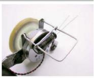
3g. Position the Solarengine circuit underneath the paper-clip frame, next to the cap, on the side opposite the motor. Solder the 3906 emitter (left) pin to the positive/anode lead of the capacitor. The connection should be short enough so that the cap holds that end of the circuit up in the air.
