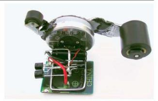
Now, put the Solarroller on a flat surface in the sun, or shine a flashlight on the cell. After a little while, the circuit will trigger, the capacitor will cump, and your Solarroller will take off for a short run. Shine, wait, and repeat.
