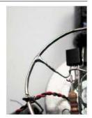
2g. Now, the solar cell. If yours has pre-tinned pads but no wires (most small cells come this way), start by soldering the 2 wires onto it - but be careful, because solar cells are fragile. Then solder the positive/red wire to the ring and the negative/black wire to the motor casing. Make the wires long enough so you can still work on the circuit, but short enough so they'll stow neatly underneath when you finally glue the solar cell down onto the ring.
