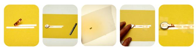
Stick a straight or fancy line of copper tape on paper. Tape a second line as close as possible to the first without touching. At the end of one line, fold the tape over on itself to create a battery switch.
