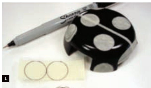
Fig. K: Building up and shaping the shell with auto body putty. Fig. L: Dime-sized masking tape circles give Beetlebot its spots.
