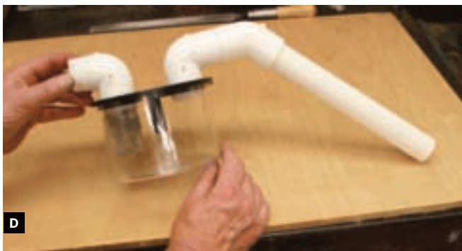
Fig. C: Glue a 2" section of pipe into the inlet elbow, and glue the 45° joint onto the other end, angled back down toward the spindle base. Fig. D: Screw the CD spindle-cover canister into place.
