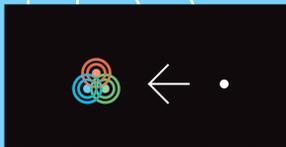
**TOO SMALL:** With a too-small pinhole, light diffraction smears the image. A smaller hole also decreases brightness, requiring longer exposures.
