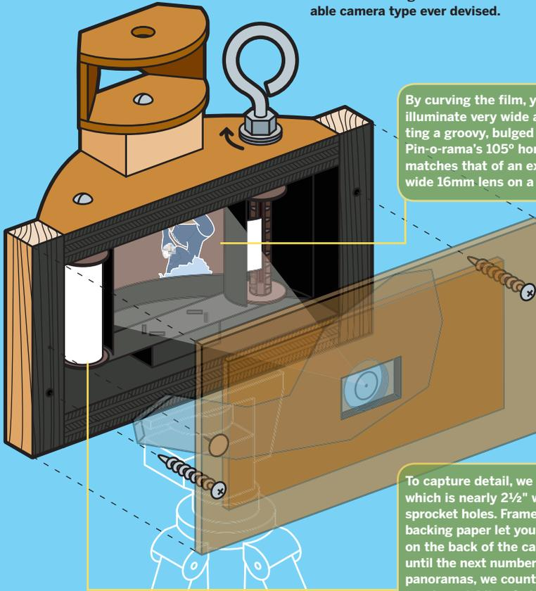
By curving the film, you can uniformly illuminate very wide angles, while getting a groovy, bulged perspective. The Pin-o-rama's 105° horizontal coverage matches that of an expensive, super-wide 16mm lens on a 35mm camera.
