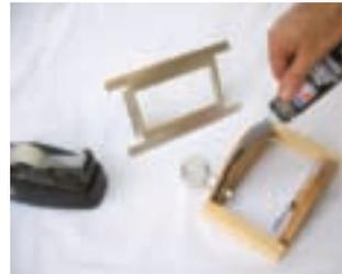
**2e.** Spread a thin bead of black silicone sealant along the plywood edges, position the film gate onto the back, and tape it into position until it cures.
