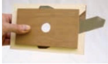
**4e.** Disassemble the pieces, and spray-paint black both sides of the inner panel, and the back sides of the shutter and outer panel. Reattach the shutter and glue everything back together.
