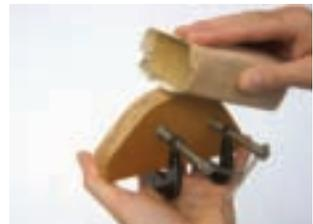
**1c.** Clamp the 2 Ds together, and sand until the cut perimeters are smooth and matching.
