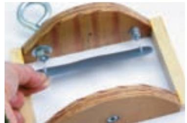
**1l.** Cut a small wooden block the same thickness as the nut stacks, and staple or tack the spring to it, centered. My block was  $\frac{3}{8}$ " $\times$ 1" $\times$ 1 $\frac{1}{2}$ ". Apply glue to the block and position it on the floor of the camera. Load the film and take-up spools between the spring nubs and the bolts, and slide the spring block around until the film spools are exactly vertical. Clamp, and let the glue set.
