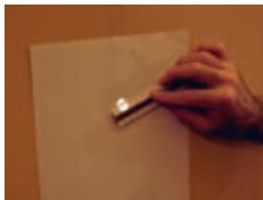
**With a projector:** Set the projector up so that a full 35mm slide image measures 52"×35". Load the pinhole into the projector, and look for the light spot to measure about 1/2" in diameter.
