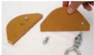
**1e.** Epoxy a ¼" #20 nut into the partial hole in the bottom piece, to make the camera's tripod mount.
