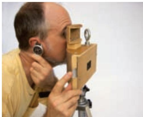
multiply the time by 150. Don't hesitate to double or triple the calculated time. Negative films are tolerant of overexposure. To time exposures without looking away from the subject, hold a watch to your ear and count ticks.
