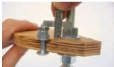
**1g.** Cut both bolt ends so each protrudes  $\frac{1}{8}$ " beyond the nut face. Get an empty 120mm film spool from a friendly camera lab, or untape one from a cheap, expired roll of 120mm film; this will be our take-up spool. File the ends of each bolt flat on 2 sides, so that they engage the slot of the spool.
