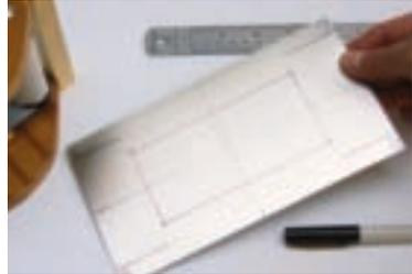
**2b.** Use tinsnips to cut along the 4 lines that extend in from the sides, and then cut the excess-overlap corners off of each piece, as marked. Then score the center rectangle lines with a sharp utility knife, and flex along the score lines to snap through the aluminum.
