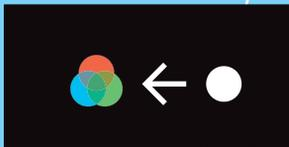
**TOO LARGE:** The pinhole's image comes from overlapping pinhole-sized blobs of light. A large pinhole loses all detail smaller than its own diameter.
