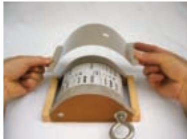
**5b.** Spray-paint black the inside of the back piece you just cut, and the interior of the camera itself. But don't paint the wooden side rails, which you'll be gluing, or the gate where it touches the film. Mask these areas with tape before spraying.
