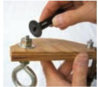
**1h.** Use thread-locking compound or mash the bolt's threads slightly to keep the nuts in place, so that the bolt assembly spins easily through the wood without loosening or tightening.
