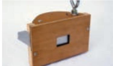
**4g.** Drill clearance and pilot holes, and use two  $\frac{3}{4}$ " wood screws to attach the front panel to the side rails, in place.
