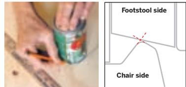
**NOTE:** You must cut the top corner radius of the chair side with a jigsaw; a circular saw would nick up the footstool side.
