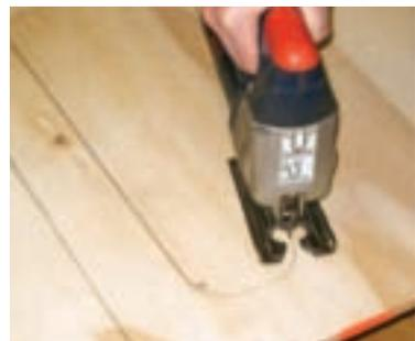
It's a good idea to use a circular saw on the straight cuts, for speed, accuracy, and to minimize sanding. Notice that the gap between plywood pieces on the layout is at least  $\frac{1}{8}$ ". Thus one cut serves 2 pieces.
