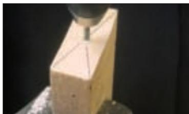
**2b.** After cutting, draw an X on all the ends of the 2x4s, corner-to-corner. At the center of each X, drill a  $\frac{5}{32}$ " hole at least 2" deep.
