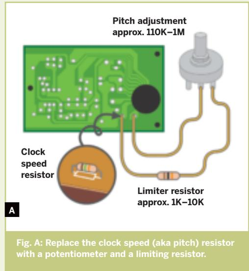
Fig. A: Replace the clock speed (aka pitch) resistor with a potentiometer and a limiting resistor.
