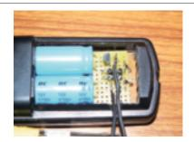
**2g.** Tie the Faraday generator temporarily to the TV remote body using cable ties, and shoot more hot glue between the remote and the Faraday tube. If you want to glue them more permanently, use a 2-part epoxy such as Araldite or J-B Weld's J-B Kwik epoxy. Now you're ready to shake!
