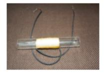
**1c.** Place the magnets inside the Faraday generator tube, stacking all 4 to make 1 big magnet. Using a hot glue gun, seal the ends with 2 pieces of perfboard, cut and filed in circular shape. To make it more permanent, use a 2-part epoxy.
