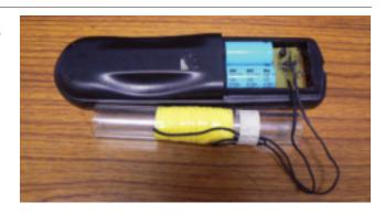
**2f.** On the remote control's original circuit board, cut down the battery terminals so that they can be soldered to the voltage regulator circuit board. Solder them to your voltage regulator output wires.
