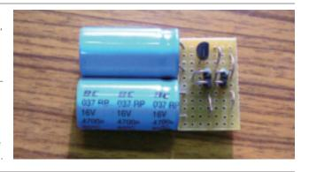
**2d.** Connect the Faraday generator. First solder 2 hookup wires in the middle of the perfboard to the input of the bridge rectifier (cathodes of diodes D3 and D4, respectively, in the circuit diagram). Then solder the wires from the Faraday generator to these hookup wires.
