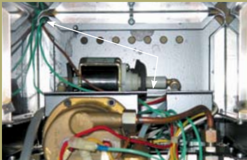
Fig. 6 Wire path out of Silvia.
