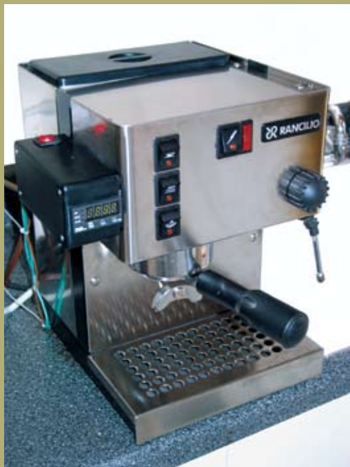
The Rancilio Silvia outfitted with temperature control.
