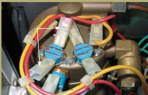
Fig. 2 Removing brew thermostat connectors.
