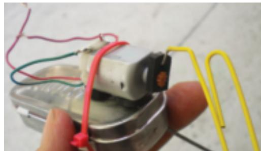
To operate the Vibrobot, twist the loose battery wire and the loose motor wire together (you can also solder an alligator clip to one of the wires for a switch). Experiment with the critter by gently bending the paper clip and legs into different shapes and observing the effects. Watch a video at [makezine.com/10/123\\_vibrobot](http://makezine.com/10/123_vibrobot).
