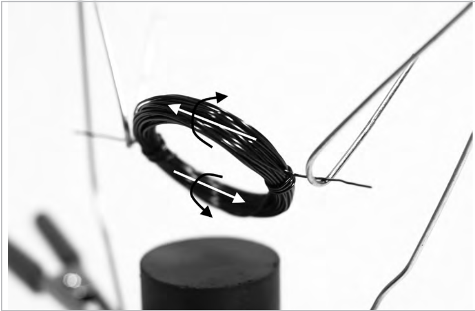
FIGURE 6-3 White arrows show direction of current flow and black arrows show the direction of the resulting magnetic field in the wire coil
